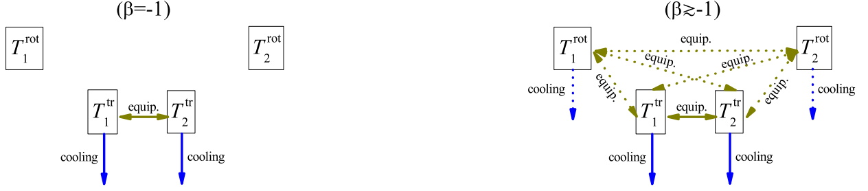
FIGURE 2. Schematic representation of the energy transfer channels in the free cooling state of a binary mixture. The left diagram corresponds to perfectly smooth particles ( \beta = -1 ), in which case both rotational temperatures are completely decoupled each other and also from the translational temperatures, so they do not change with time. The right diagram corresponds to quasi-smooth particles ( \beta \gtrsim -1 ), in which case weak channels of energy transfer exist and also the rotational temperatures are subject to a weak cooling.
